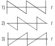
a) Which curve do you get from this output signal 1 when you use the switch at the mixer which shows the following sign  $\emptyset$ ? b) What does this sign mean?
