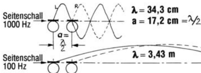
$\Delta \varphi = 180^\circ$ ; Korrelationsgrad  $\cos \varphi = -1$
